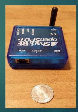
When a SharkRF openSPOT is connected to an inexpensive portable router (tp-link) and smart phone Hot Spot, a Ham can use their HT literally anywhere in the world through the internet.
