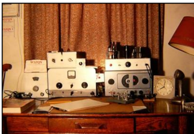
Bob's shack in 1957- Heath VF-1 VFO, Heath AT-1 Transmitter, with a Heath tuner on top, Hallicrafters S-38C Receiver with a home brew modulator on top.
