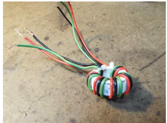
Completed Ferrite Torrid
