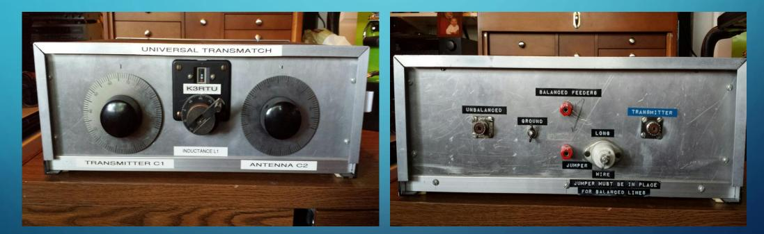
WIDE CAPACITOR PLATE SPACING GIVES THIS DESIGN THE ABILITY TO HANDLE WELL OVER THE LEGAL POWER LIMIT. VERNIER DRIVES AND A TURNS COUNTER MAKES TUNING PRECISE AND EASILY RESET WHEN CHANGING BANDS.
