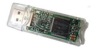
The Amateur Radio research organization TAPR produced a vocoder using the AMBE-1000 device in 1999.
