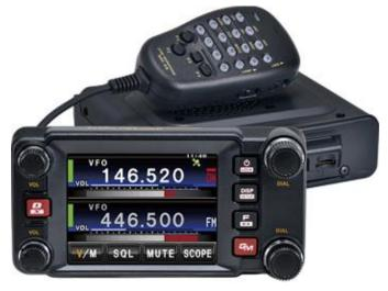
But the System Fusion II digital voice protocol at 7.2 kb/sec uses C4FM (Continuous Four Level Frequency Modulation) for a transmission bandwidth of 12.5 kHz, lower than the 28.8 kHz expected.
